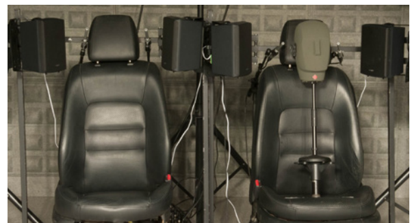
Figure 2. Car seats with transducers.
