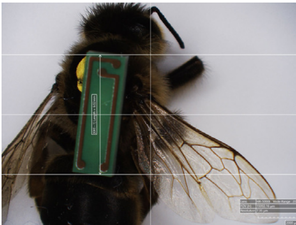
RFID chip antenna used to detect queen bees in a honeycomb (INNDeAPI project).
